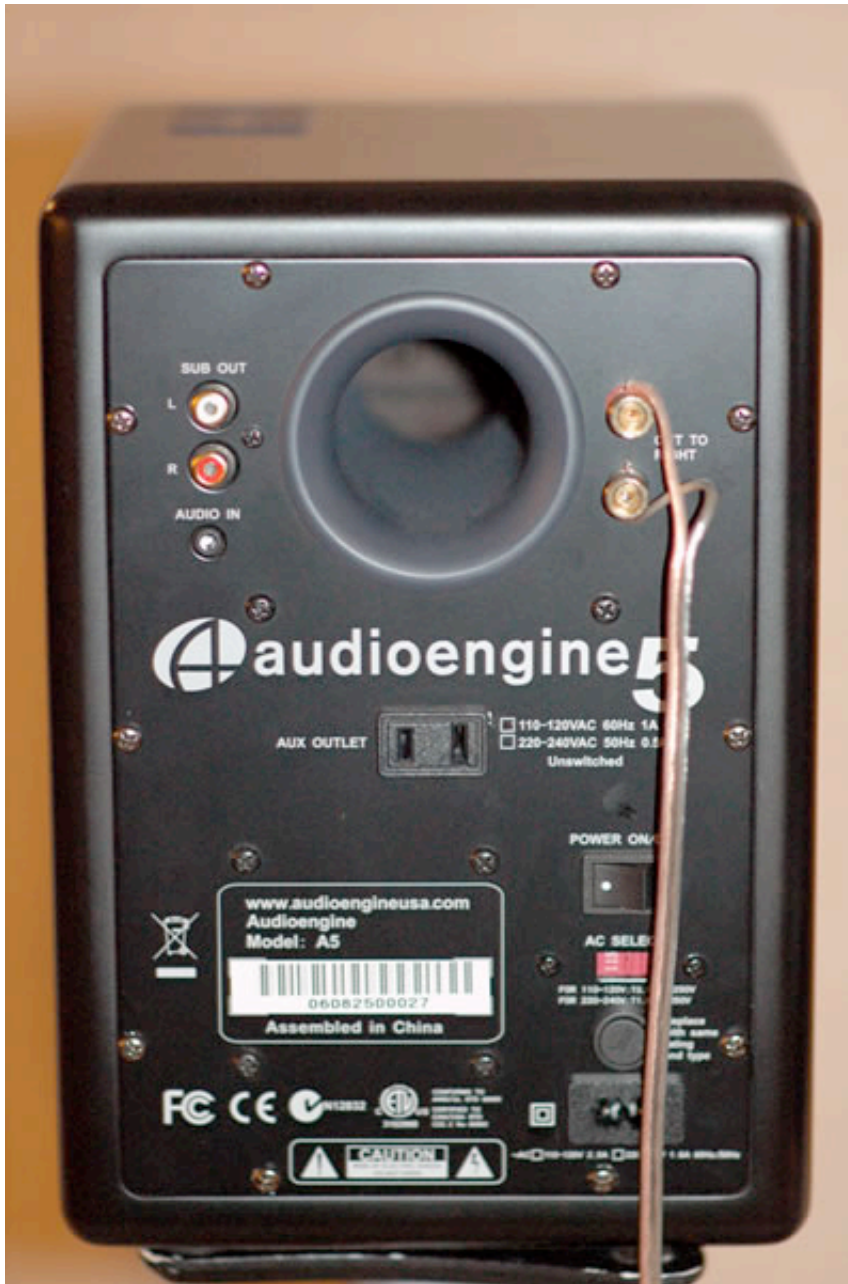
The back plate of the left A5, which has the power supply and ports.
